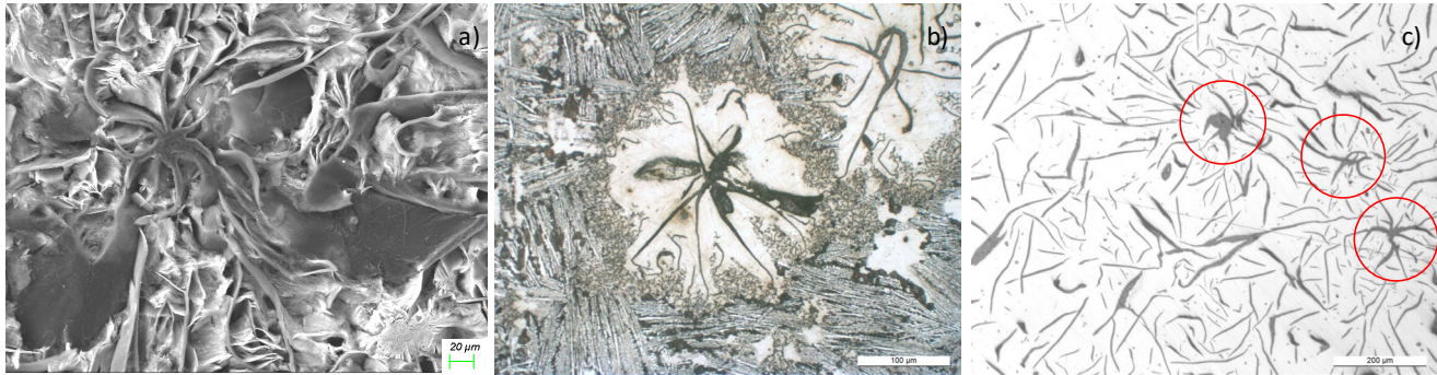
Figure 6. Presence of kish graphite on samples without niobium; a) deep etched SEM micrograph showing the branching of the kish graphite; b) quenched sample with a solid fraction of 0.35 calculated by the method described in Reference 24; c) thermal analysis cup, where the kish graphite was identified by red circles.
